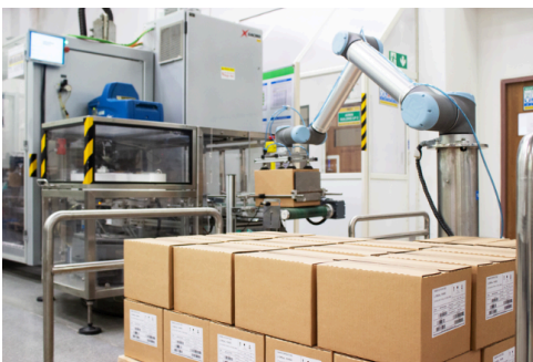
Palletizing as a typical pick & place scenario
